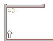
yoke beams. If you press the left mouse button in this moment, this point is taken as starting point. This starting point is shown as a black arrow. If you do not click with the mouse on a sketched arrow, the selection of a starting point is deleted. For a calculation at the end all kinds of solutions are calculated.
