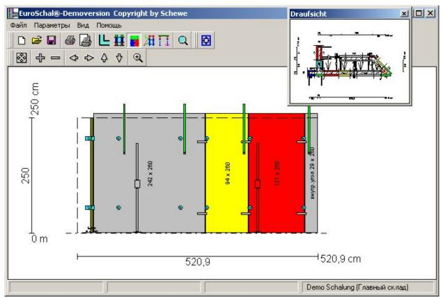
On the screen the side view of a wall is shown in large format. The view is shown in a small window the right corner. This window can be shifted and changed in size.
