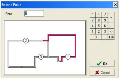
When inserting objects (view, material list...) the pour selection window is always shown when the floor plan is divided into pours. Mark the one you need with the mouse.
